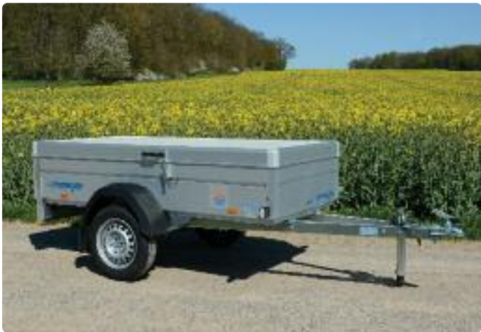
HZ 7521/106 Zubehör: Stützrad, Sandwichaludeckel HZ 7521/106 Options : roue jockey, hardtop en aluminium sandwich HZ 7521/106 Optional extras: jockey wheel, sandwich aluminium hardtop
